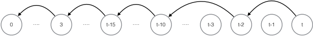
Figure 1: Recovering backward chain from time t : t_0 = t, t_1 = t - 2, t_2 = t - 10, \dots, t_5 = 0 . Here, H(t) = 5 .
